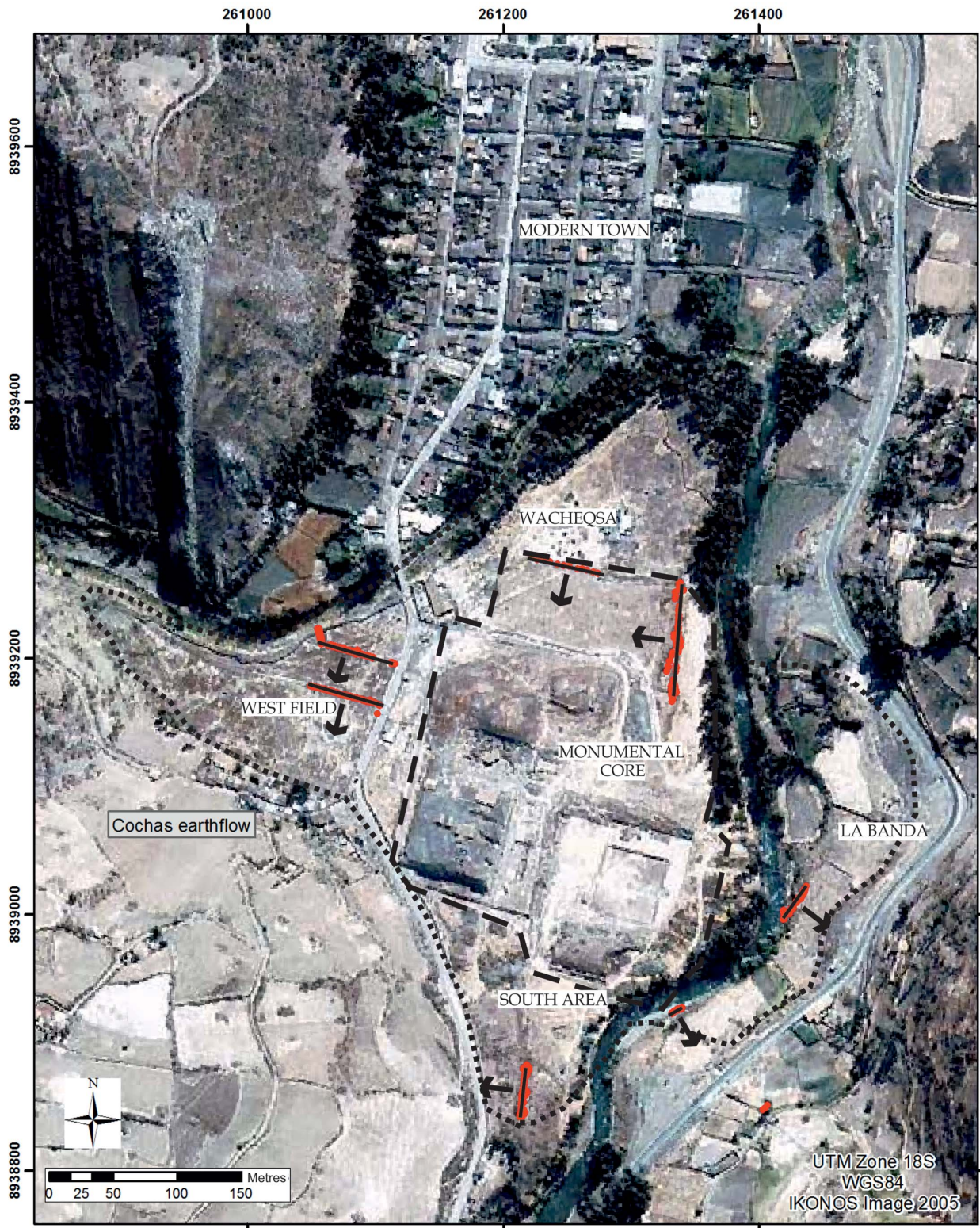
Figure 3. (Colour online) Landscape engineering surrounding the site core. Wall fragments indicated are either platform facades or retaining walls; black arrows indicate direction of retention and presence of at least partially artificial fill. The approximate extents of the monumental core and the modified landscape are indicated by the dashed and dotted lines, respectively. The fin of quartzite north of the West Field is the Shallapa outcrop, likely source of much of the site's building stone.
